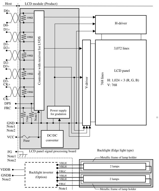
Note1: Connections between GND (Signal ground), FG (Frame ground) and VBLC (Lamp low voltage terminal) in the LCD module
